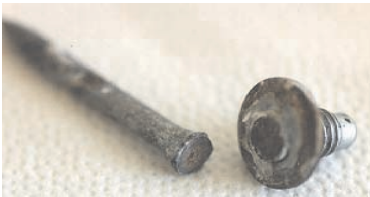
Fig. 13: These galvanised nails were used in a corrosive industrial environment. The cause of failure was secondary (corrosion-induced) hydrogen embrittlement.
