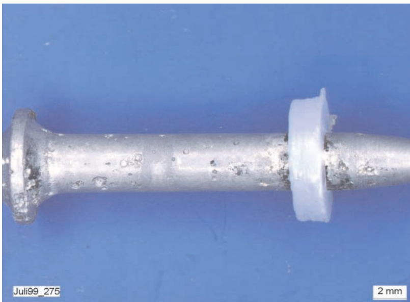
Fig. 6: Pitting of a fastener made of the 1.4301 (AISI 304) material (Competitor Product)
