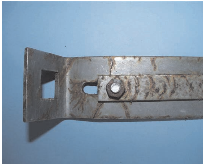
Fig. 12: This shows SCC of a retaining strap made of the material 1.4301 (A2, 304) after approx. 4 years of use in an indoor swimming pool (CH)
