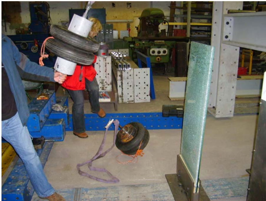
Test piece 3 Impact on P1 to test the residual load-bearing capacity; height of drop \Delta h = 100 m → no further damage
