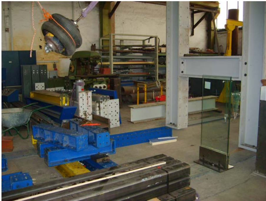
Test piece 1 Impact on P1 from a height of drop of \Delta h = 900 m → no damage
