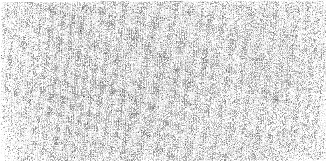
Fig. 6: Micro-section (etched) of 316L specimen material; longitudinal micro-section (200 x magnification)
