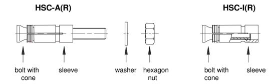
Installed condition: HSC-A(R) safety anchor (externally threaded version)
