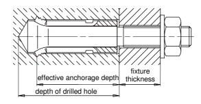
Installed condition: HSC-I(R) safety anchor (internally threaded version)
