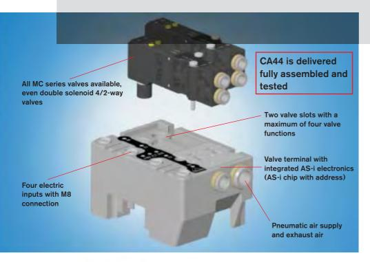
Extremely adaptable and efficient-CA44 is the intelligent solution for integrating pneumatic valves in systems with AS-i bus structures:
