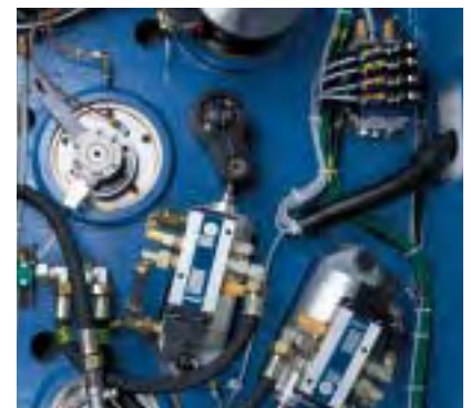
Cylinder valve units for turning the impression cylinders on and off.
