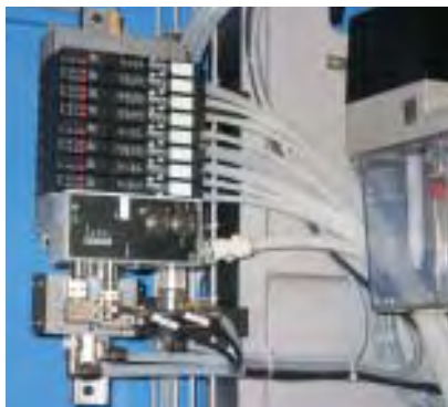
Actuator (cylinder) controlled by the HF03 valve terminal system with a bus connection.
