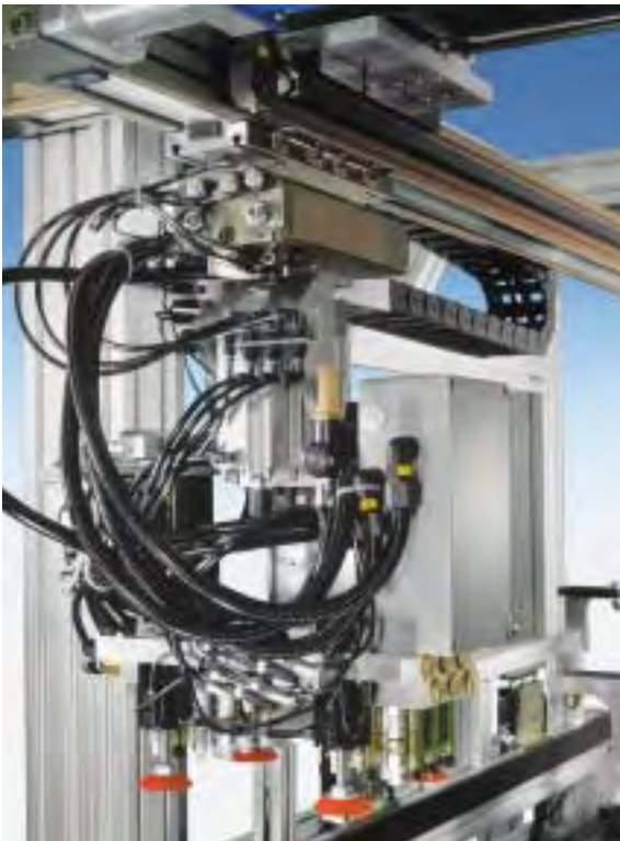
Rexroth's shuttle cylinder, RexMover, is used to load the tortilla bread boxes carefully and efficiently on the pallet.
