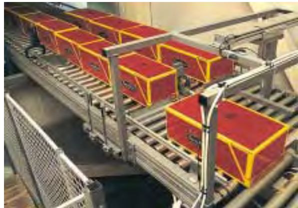
Rexroth's shuttle cylinder, RexMover, is used to load the tortilla bread boxes carefully and efficiently on the pallet.
