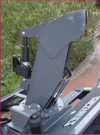
▲ Deflector superior ajustable eléctricamente Adjustable upper deflector electrically
