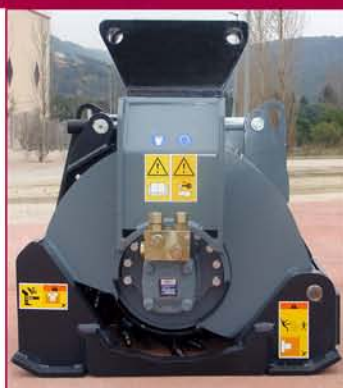
▲ Soporte basculante que permite fresar en cualquier superficie (horizontal, vertical e inclinada) Swinging suport that allows to plane and cutting any surface (horizontal, vertical and inclined)
