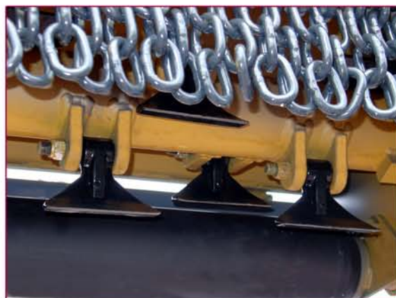
▲ Detalle martillos Detail hammers
