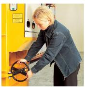
A threaded spindle ensures steady and safe opening of the main door
