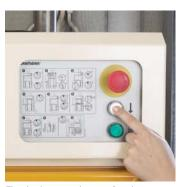
The bale press has a simple control panel and is equipped with easily understood pictograms.
