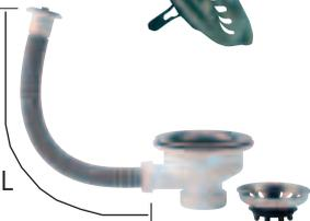
B-72-113    | 1000421 | <ul style="list-style-type: none"> <li>rebosadero vertical redondo con chapa</li> <li>tubo flexible</li> <li>chapa cesta inox. Ø113-Ø84</li> <li>chapa rebosadero inox. Ø37,5</li> <li>salida 1 1/2=Ø40</li> <li>L: 320 mm</li> </ul> |
