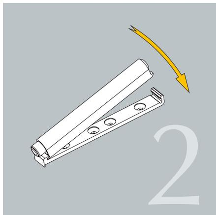
PRESSIONAR EL CUERPO DE LA PARTE TRASERA DE LA BASE HASTA FIJARLO.
