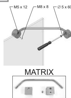
The product is for mounting in a totally finished (tiled, plumbed, etc.) bathroom and fitted shower tray (if used). The constructional dimensions and/or shower tray dimensions must be in strict accordance with the dimensions of the selected shower door or enclosure i.e. nominal 80, 90, 100, 110, or 120 cm. according to type. For best results, the product must only be fitted to a strong and rigid, solid bathroom wall that is vertical and adjacent walls should be square to each other.
