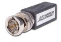
The American Dynamics ADACTP01BNC Twisted Pair Video Adapter is a passive transmission device that transmits video or video with up-the-coax (UTC) dome control signals over unshielded twisted pair (UTP) cables, point-to-point, for distances up to 300m (1000 ft).
