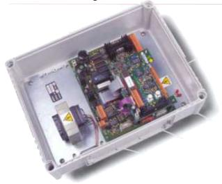
For use within the most sophisticated CCTV surveillance systems, the Synectic Systems DCRXP\*1 telemetry receiver offers maximum operational control of variable speed DC pan and tilt heads, lenses and fast pre-set positioning.
