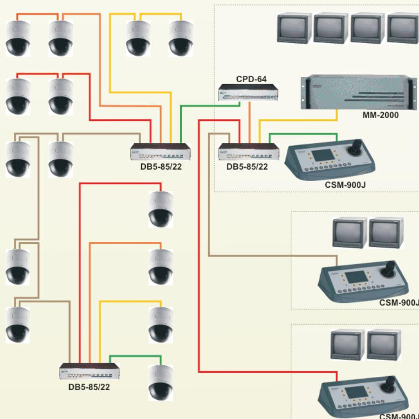
Application example in a matrix system OMIKRON, with domes, with three control points, united by means of independent communication buses.
