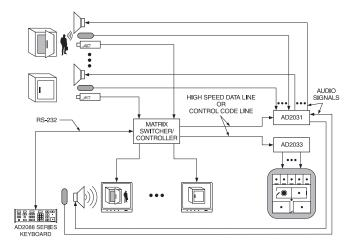
SPEAKER & MICROPHONE OR OTHER AUXILIARY EQUIPMENT ACTIVATED BY AD2031 RESPONDING TO CAMERA CALLUP TO MONITOR GRAPHIC DISPLAY PANEL OR OTHER AUXILIARY EQUIPMENT ACTIVATED BY AD2033 RESPONDING TO AUXILIARY COMMAND
