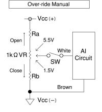
\*Vcc represents Input Voltage. \*The Remote Voltage should be set between 1.5~5.5V, and Level remote should be OFF.
