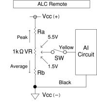
\*Vcc represents Input Voltage. \*The ALC should be set at the full Pk position. 3)Over-ride Manual T34Z5518AMSR-CS/AMSPR-CS H16Z7516AMSR/AMSPR (IR) H30Z1015AMSR/AMSPR
