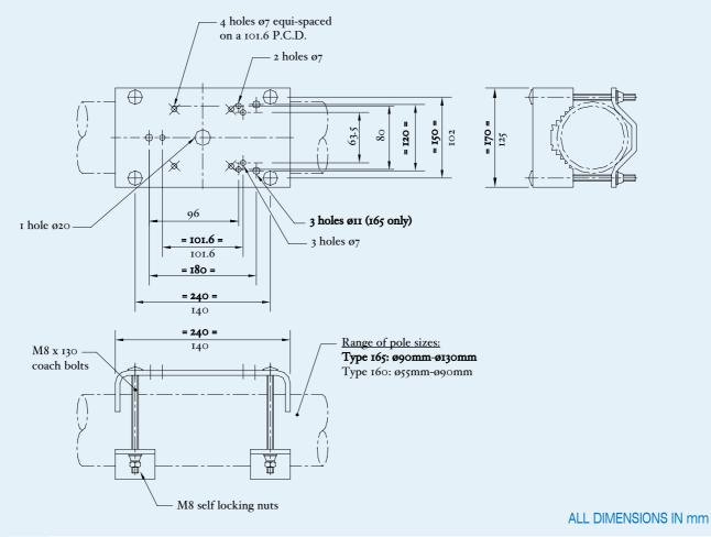
SPECIFICATION **Type 160** Type 165 Material Mild steel Mild steel Finish Zinc plated and painted Zinc plated and painted Maximum load 15kg 25kg PAYLOAD OPTIONS 428 bracket 428 bracket 642 bracket 508 housing 508 housing 554 dome 554 dome 556 dome 556 dome 2010 housing 2010 housing 2050 dome 2050 dome
