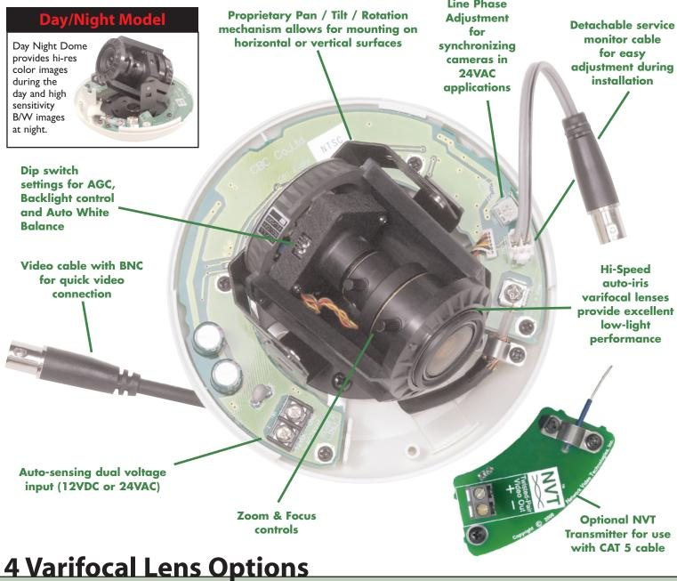
Integrated **computar** auto-iris varifocal lenses provide a wide variety of adjustment ranges.
