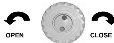
Turn the outer ring a quarter anti-clockwise to open the jet.
