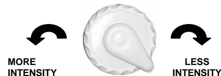
The jets can also adjust the flow intensity when opening and closing the water. To do this, proceed as follows:
