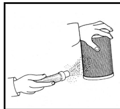
5. After several washing cycles, it may be necessary to change the filtering cartridge.
