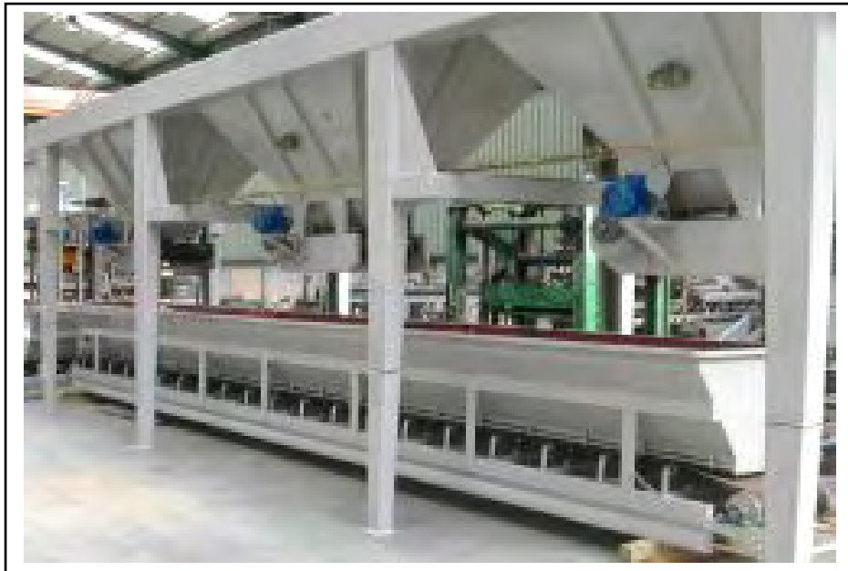
Conos tolvas + Cinta pesadora / Cones for hopper + Weighing band
