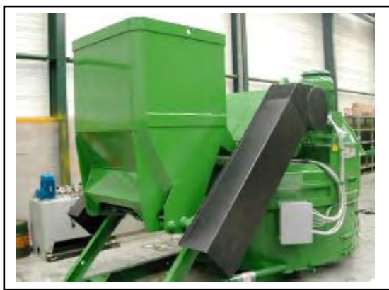
SKIP INCLINADO / SKIP INCLINATED
