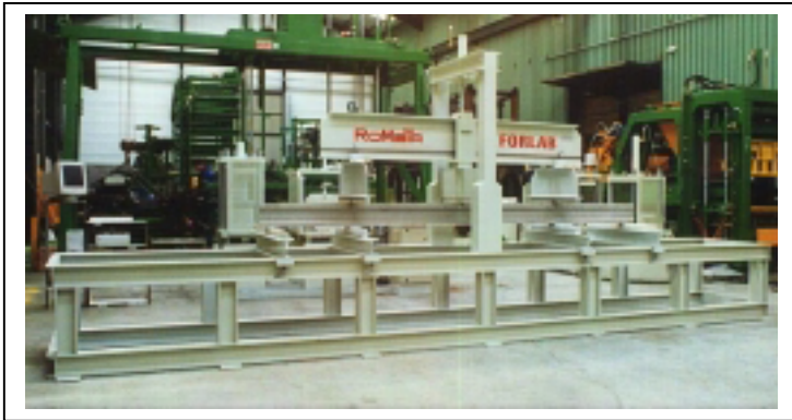
Tolvas aéreas / Concrete transport shuttles
