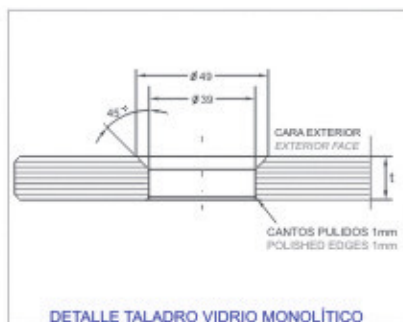
DETALLE TALADRO VIDRIO MONOLÍTICO MONOLITHIC GLASS HOLE DETAIL
