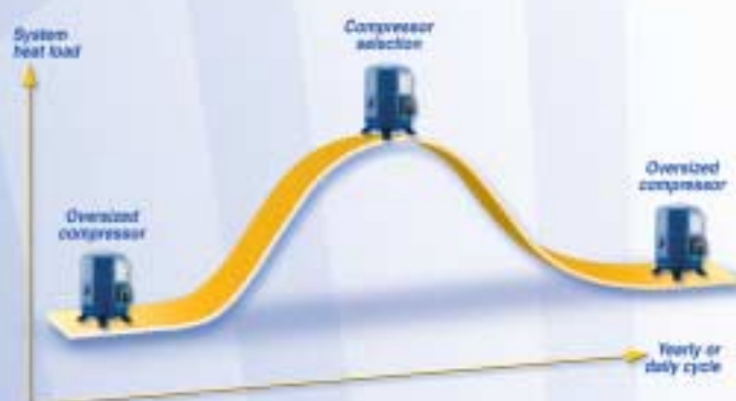
Typical system load profile
