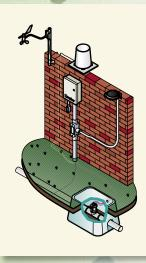
Data Retrieval Units report flow, rain, wind, and other conditions from sensors. This real-time feedback makes it possible to monitor and react to alarm situations when detected.
