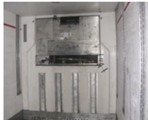
▲ Bad cooling in trailer: IR shows that discharge opening is blocked on the left side
