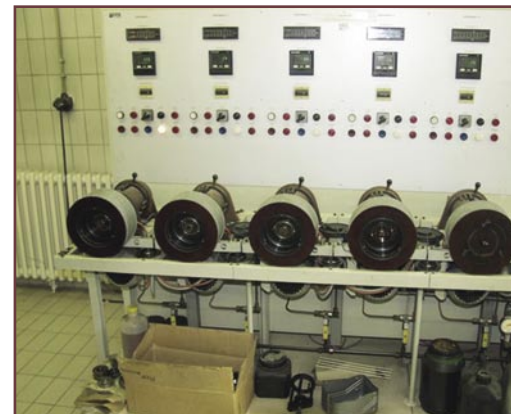
◆ Bearings on FAG FE9 test bed, ThermaCAM E-series linked to laptop
