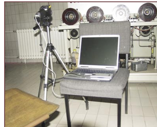
◆ Bearings on FAG FE9 test bed, ThermaCAM E-series linked to laptop
