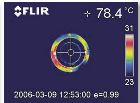
Heat development of new and old bearing, showing increased heat on outer ring
