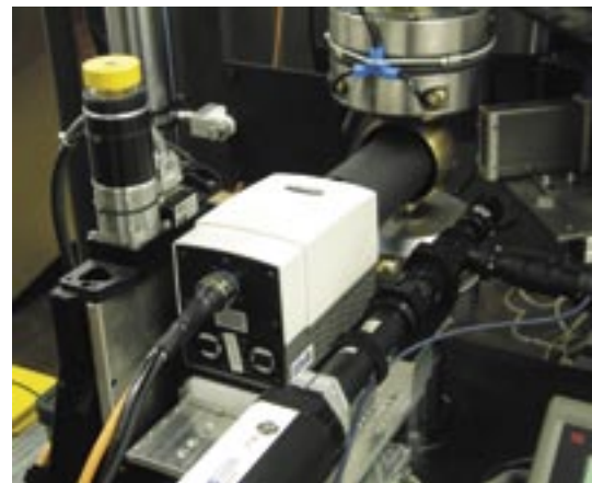
Phoenix IR camera placed on testbed, specimen is covered by messing sphere for thermal shielding
