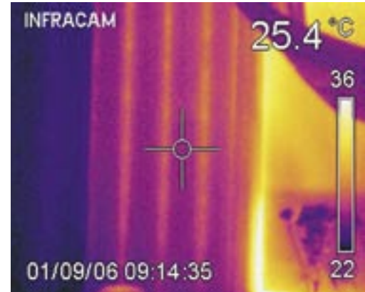
The image clearly shows where not to drill.
