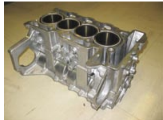
Cylinder bloc manufactured at the Cléon plant
