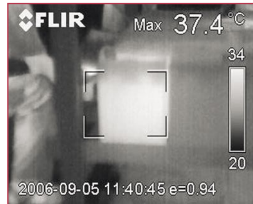
◆ UPS Battery block: a battery needs to be replaced
