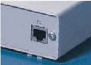
Interface for linking the sensor unit and processing unit. Used for data transmission and power supply. Cable 7320.470/.472/.481.
