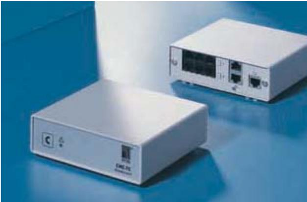
This sensor unit allows the remote release of one or two door systems for access via the network, as well as the initiation of personalised opening via a read system (smart card reader). The system also monitors the status of the door, handle or latch. Authorised access codes can be set up via http. The sensors/actuators/readers listed below can be operated here.
