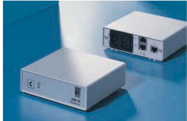
A temperature control circuit is installed with this sensor unit. Temperature setpoints are set via the PU, and these are then compared with the actual temperature. Depending on the evaluation, the fan system is activated. The function of the fans can also be monitored with an airflow sensor. Monitoring is only active with the fan operational. Other sensors may optionally be connected to the unit.
