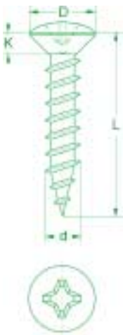
CABEZA GOTA SEBO PHILIPS ROSCA MADERA DOBLE HILO PHILIPS RAISED COUNTERSUNK HEAD DOUBLE THREAD WOOD SCREW VIS A BOIS A DEUX FILETS TÊTE FRAISÉE BOMBÉE PHILIPS
