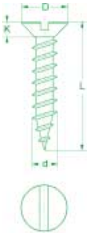
CABEZA PLANA RANURA ROSCA MADERA DOBLE HILO SLOTTED COUNTERSUNK HEAD DOUBLE THREAD WOOD SCREW VIS A BOIS A DEUX FILETS TÊTE FRAISÉE FENDUE
