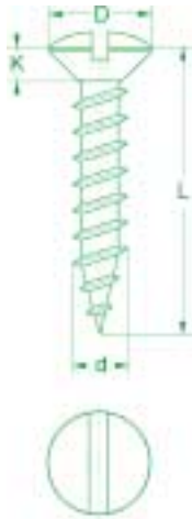
CABEZA GOTA SEBO RANURA ROSCA MADERA DOBLE HILO SLOTTED RAISED COUNTERSUNK HEAD DOUBLE THREAD WOOD SCREW VIS A BOIS A DEUX FILETS TÊTE FRAISÉE BOMBÉE FENDUE
