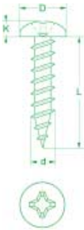
CABEZA ALOMADA PHILIPS ROSCA MADERA DOBLE HILO PHILIPS PAN HEAD DOUBLE THREAD WOOD SCREW VIS A BOIS A DEUX FILETS TÊTE CYLINDRIQUE BOMBÉE LARGE PHILIPS
