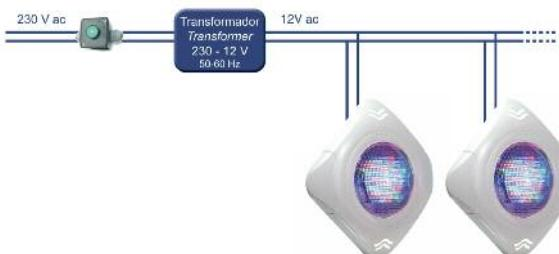
Basic LT wiring from a standard 12V AC transformer. Push-button control. The synchronizing signal for color change and access to in-built programs travels through the power cables.
