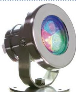
AdLed Mini Adjustable Projector are a range of fixtures to light statutory, architectural features and other elements in wet environments. Manufactured in AISI316 stainless steel. Available with wide, medium and narrow angle optics. IP68.
