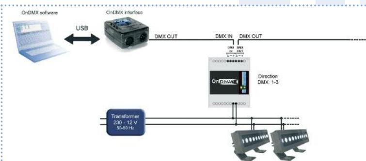
For absolute control, DMX 512 wiring permits independent addressing of each fixture, millions of colors and infinite sequences.
