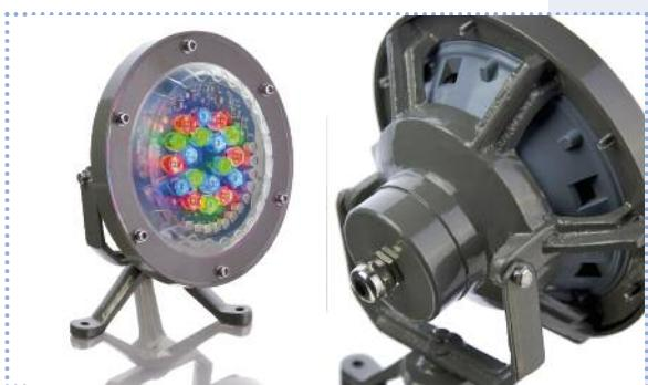
Directional fixture for PAR56 lamps in cast light alloy with epoxy anti-corrosion finish and stainless steel fasteners. Supplied with cable. Does not include lamp. For waterworks and fountains. IP68.
