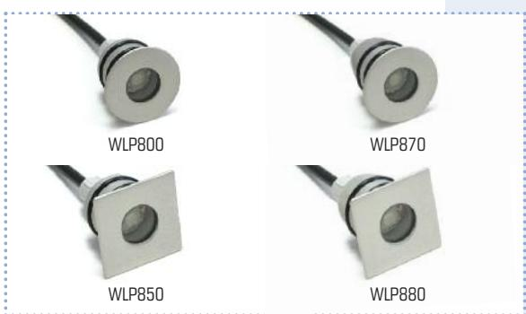
Miniature fitting for installation on floors or walls. Manufactured from light alloy. Snug fitting with o-rings in standard Ø40mm PVC tubes. Available with wide, medium and narrow angle optics.
