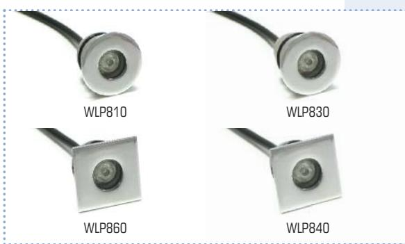
Miniature fitting for installation on floors or walls. Manufactured from AISI316 stainless steel. Snug fitting with o-rings in standard Ø40mm PVC tubes. Available with wide, medium and narrow angle optics. IP68.
