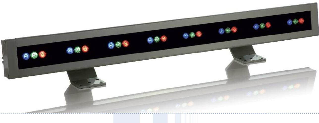
AdLed linear projectors, manufactured from light alloy with epoxy protective finishes. Available in different whites and single colors with a range of optics including elliptical configurations for wallwashing. Also available in RGB, for LT or DMX control. Temperature operating range -10° to +65°C. Delivered with 3m power cord. Burial boxes in AISI316 stainless steel for flush installation on floors and walls available on request. IP68.
