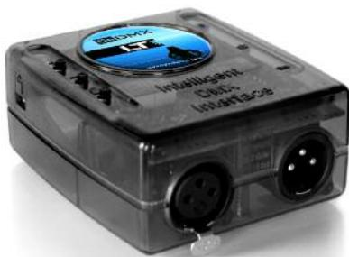
DMX Modulator to act as interface between the controller and the AdLed fixtures. One modulator is required for each group of fixtures sharing the same power supply.
