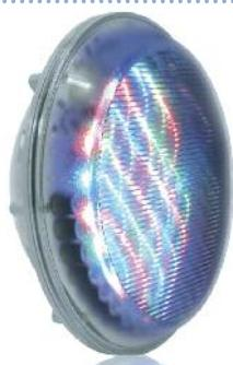
AdLed PAR56 12V AC lamp with a choice of medium or narrow-beam optics. Built in electronic circuits with programs in RGB models for color change and sequences. For waterworks and fountains. IP68.
