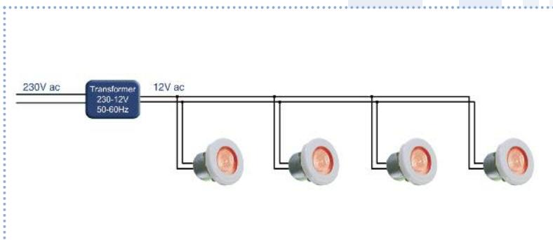
Single color AdLed Mini wiring from a standard 12V AC transformer.
