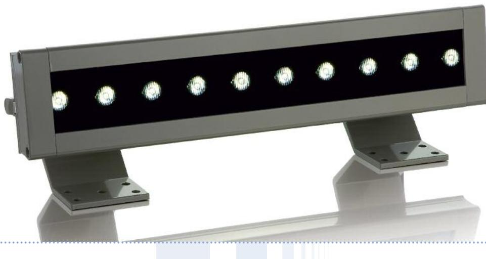
AdLed linear projectors, manufactured from light alloy with epoxy protective finishes. Available in different whites and single colors with a range of optics including elliptical configurations for wallwashing. Also available in RGB, for LT or DMX control. Temperature operating range -10° to +65°C. Delivered with 3m power cord. Burial boxes in AISI316 stainless steel for flush installation on floors and walls available on request. IP68.
