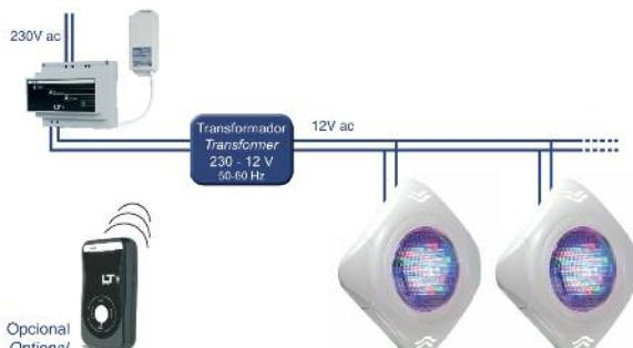
RC-LT wiring from a standard 12V AC transformer. Remote control. The synchronizing signal for color change and access to in-built programs travels through the power cables.
