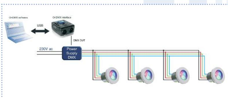
For absolute control, DMX 512 wiring permits independent addressing of each Mini fixture, millions of colors and infinite sequences.
