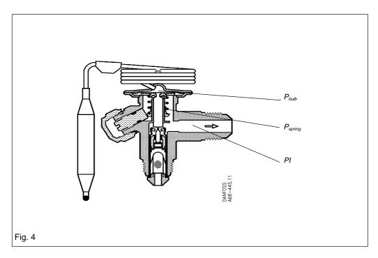
The valve function is controlled by the intermediate pressure (PI) acting under the diaphragm and the bulb pressure derived from
